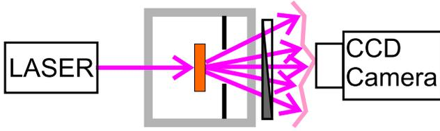
FIG. 1 (color online). The experimental setup. The sample is placed in a pressurized chamber and illuminated by a HeNe laser. A single polarization of the transmitted speckle is recorded by a CCD camera.
