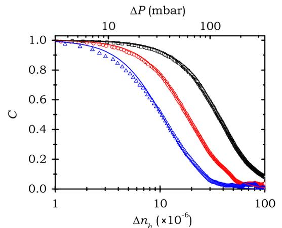
FIG. 2 (color online). RIT autocorrelation coefficient as a function of  $\Delta n_h$ . Data points show measurement results for 3 slabs of polyethylene filters ( $L = 1, 1.5,$  and  $2 \text{ mm}$  for black squares, red circles, and blue triangles, respectively). The lines show the fit to theory [Eq. (5)].
